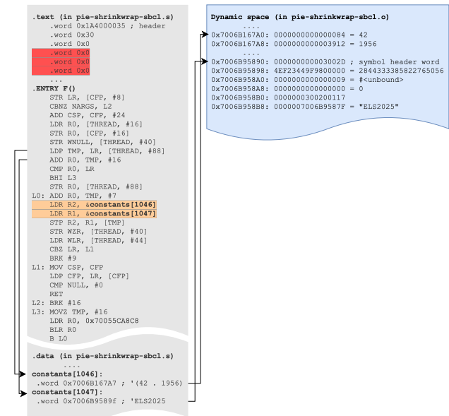
Figure 4: Representation of the same code object and the cons and symbol objects it references after code/data segregation and the rest of the shrinkwrapping process.
