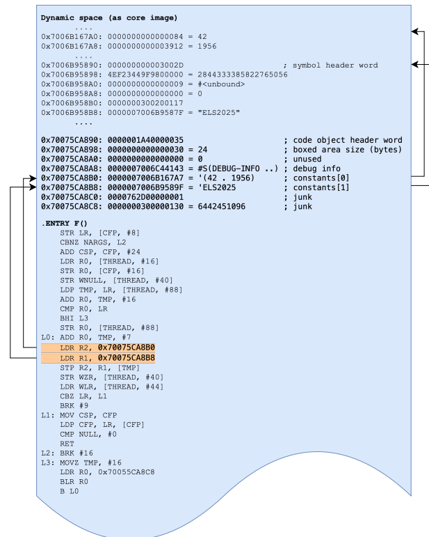
Figure 3: Representation of the compiled code object (in boldface) for the function #'f in memory, along with the cons and symbol objects it references.
